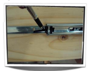
When the end of the plastic lever is pointing down, then move your finger towards the back of that lever and depress it down.
